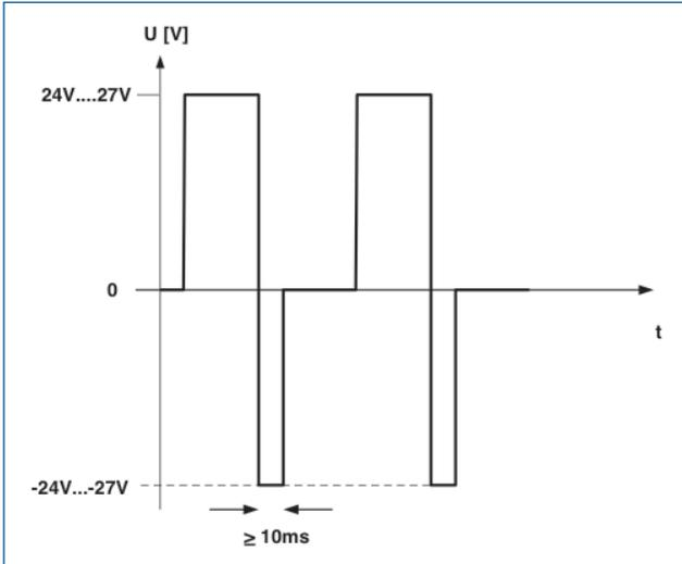
The physical characteristics of piezo ceramics under electrical voltage or temperature will cause a drift (relaxation) of the factory set switch on/off voltage. To avoid negative influence on the smart positioner function we strongly recommend to use the following piezo specific electrical control.
